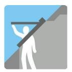
A top-hung roof window with bottom operation is ideal if you have to, or wish to, place your window in a high position, for instance in connection with a high knee wall.
